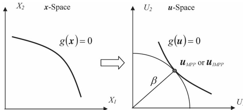
Figure 1. Transformation of input variables and illustration of most probable point (MPP).
