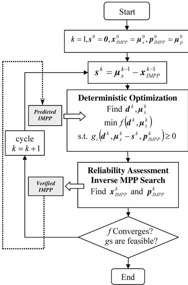
Figure 2. Flowchart of the original SORA method.
