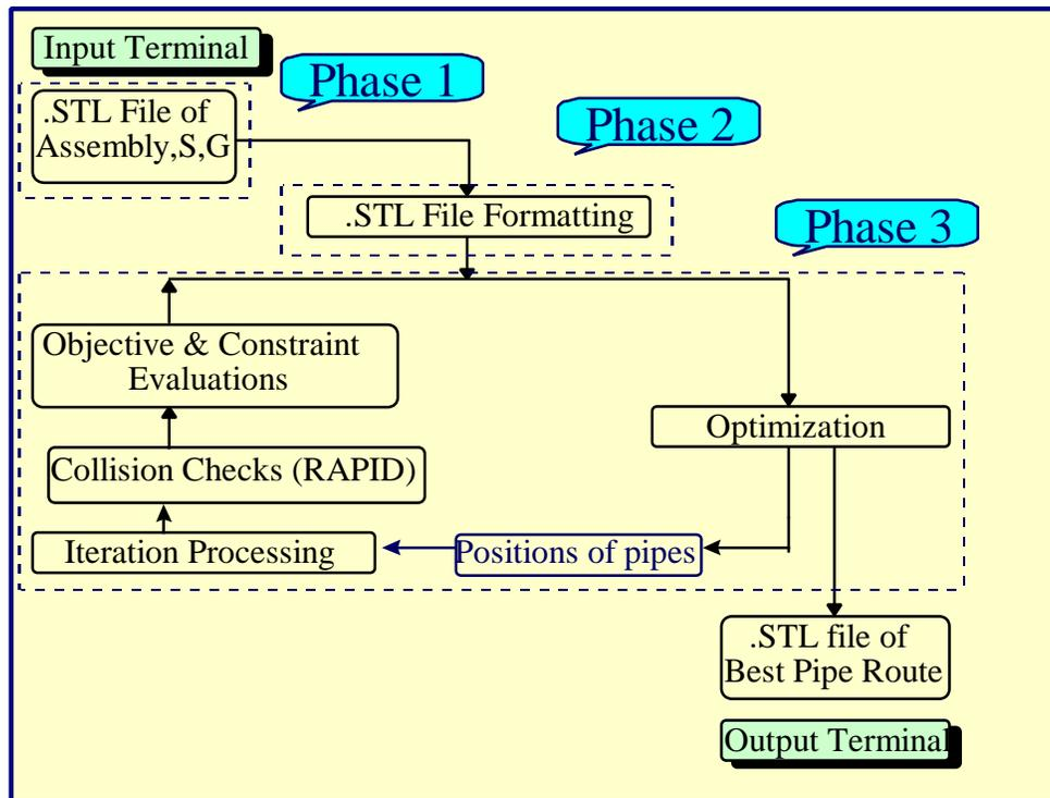
Figure 3. GAPRUS PIPE ROUTING PROCESS FLOW CHART
