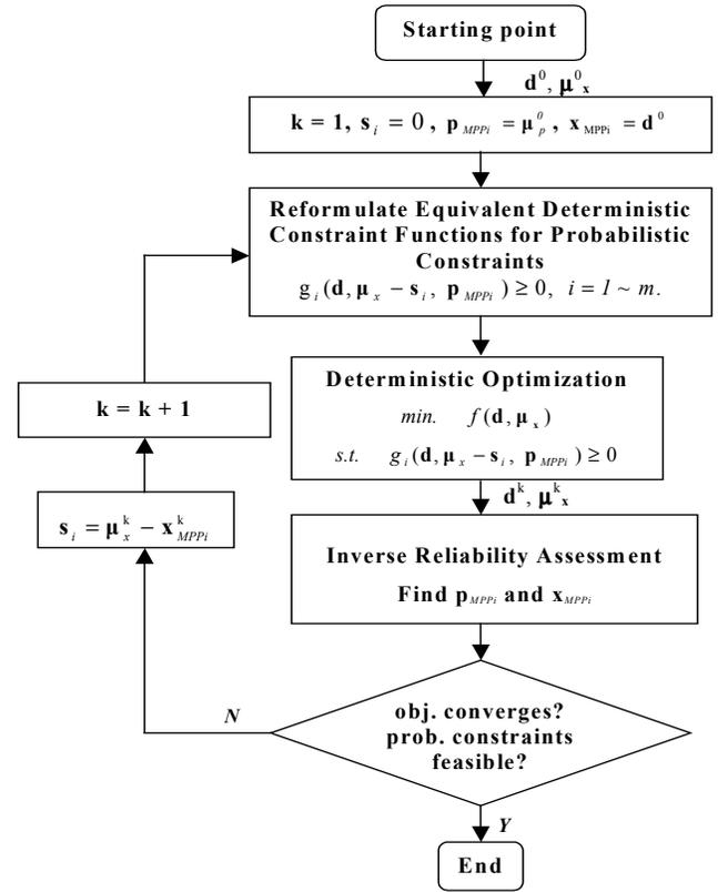
**Figure 3. Flowchart of the SORA Method**
