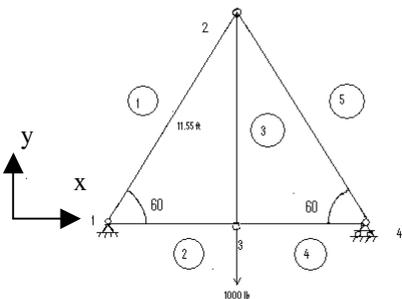
Figure 6. 5-bar Truss
