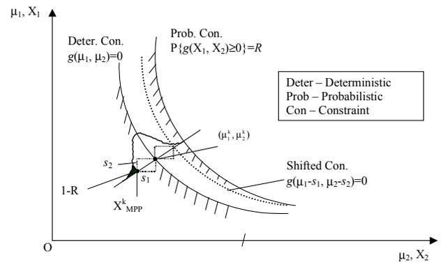
**Figure 4. Shifting Distance of Probabilistic Boundaries [4]**
