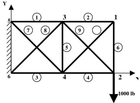
**Figure 8.** 10-bar Truss
