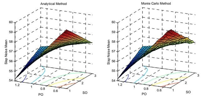
Figure 12b. Mean of Slap Noise Evaluated by Analytical Method (left) and Mean of Slap Noise Evaluated by Monte Carlo Method (right).
