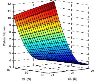
Figure 8. Interaction Between CL and SL for Piston Friction
