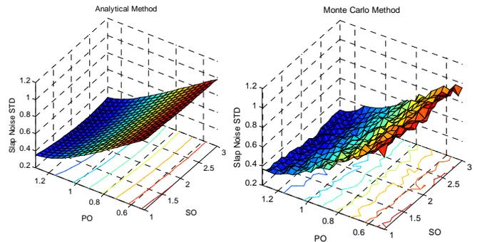
Figure 13a. STD of Slap Noise Evaluated by Analytical Method (left) and STD of Slap Noise Evaluated by Monte Carlo Method (right).
