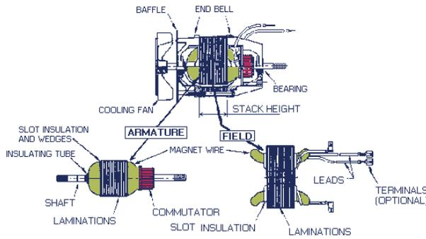
**Figure 9. Universal Motors Schematic**
