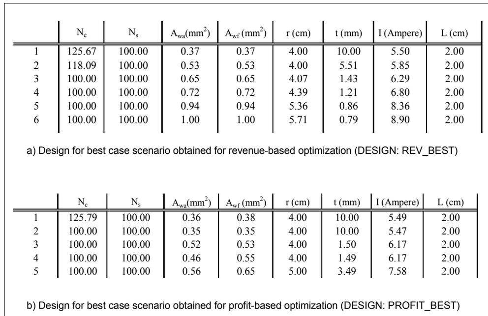
**Figure 14. Comparisons of Motor Designs Obtained Using Revenue- and Profit-Based Optimization**
