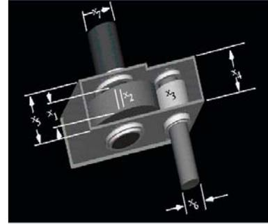
Figure 7. The speed reducer of a small aircraft engine
