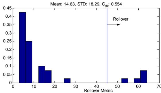
**Figure 2. Rollover Metric Distribution for Baseline Design**
