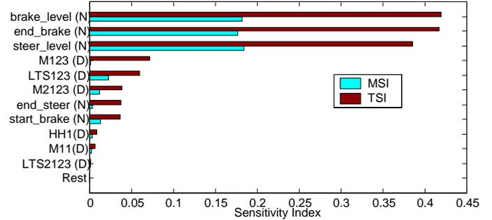
Figure 3. Sensitivity Indices of 19 Variables (D-Design Variable, N-Noise Variable)
