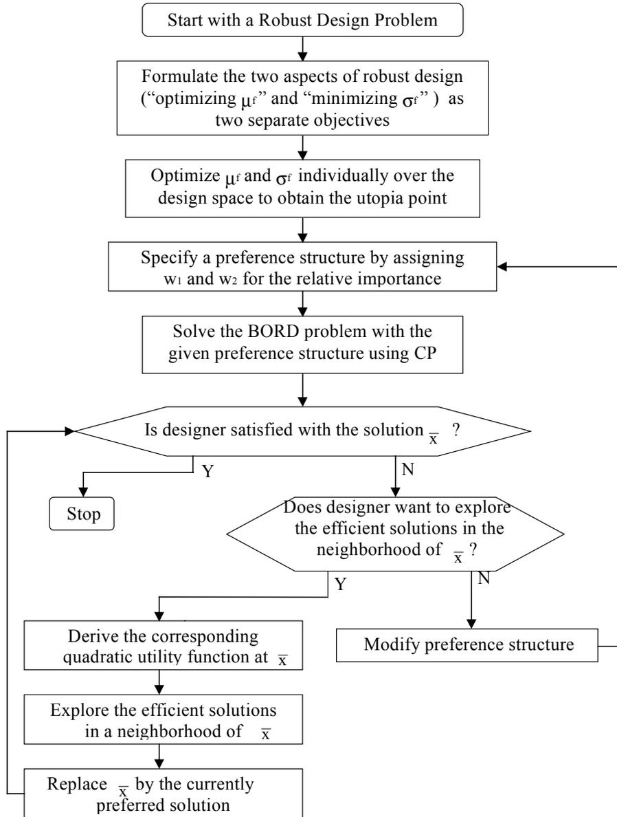
**Figure 1 A Robust Design Procedure for Addressing Multiple Aspects of Robust Design (Chen et al. 1998)**
