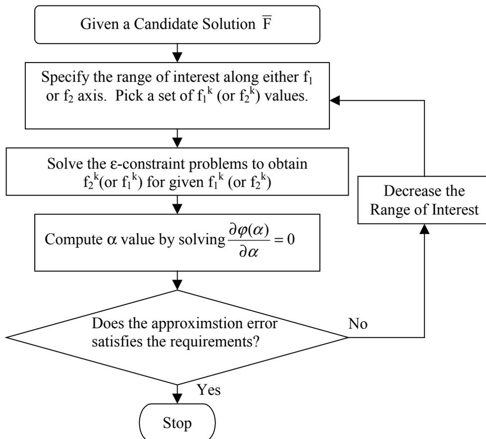
**Figure 4. A General Procedure for Determining Parameter  $\alpha$**
