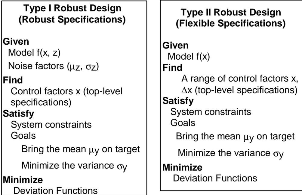
Figure 2. Two Types of Robust Design
