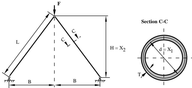
**Figure A.1 The Two-Bar Structure**
