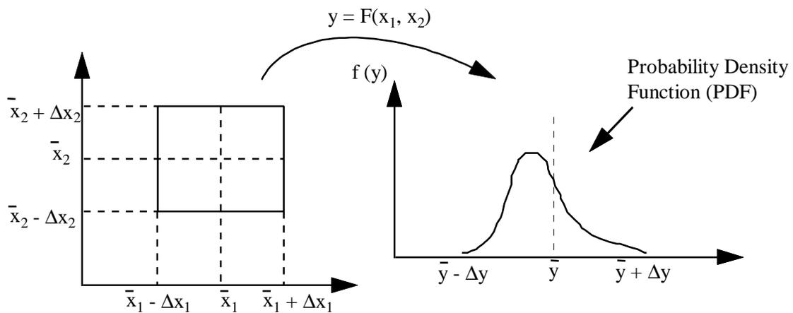
**Figure 2 Mapping between Design Variables and Design Performance**
