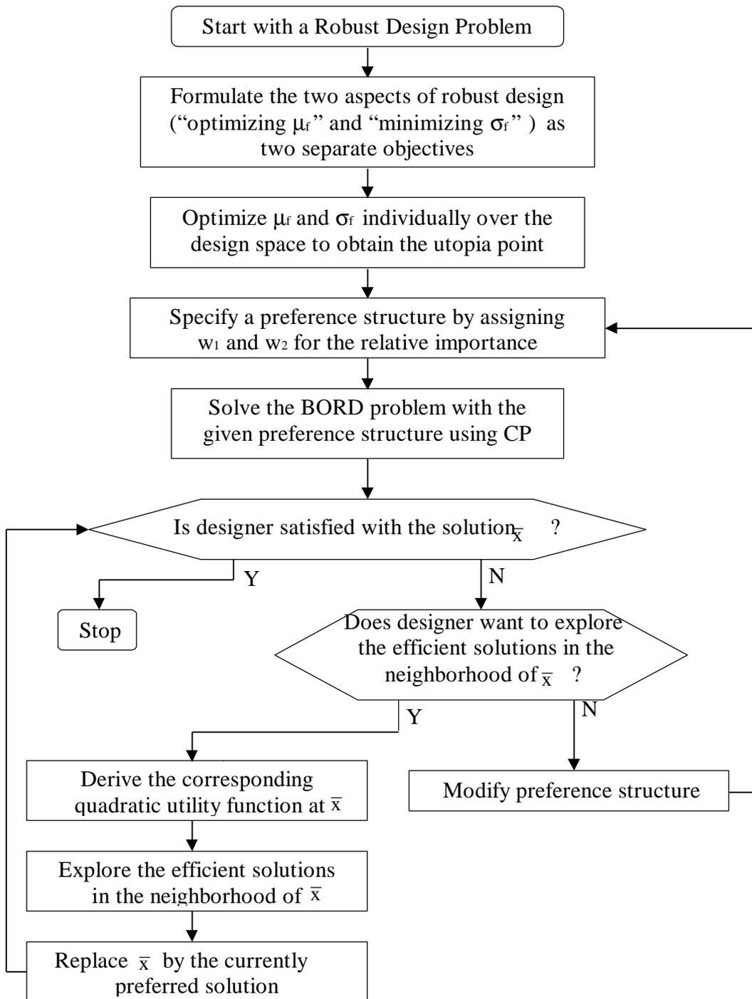
**Figure 4** A Robust Design Procedure for Addressing Multiple Aspects of Robust Design
