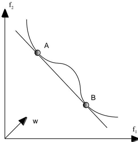
**Figure 2 Generating Efficient Solutions by the WS method**
