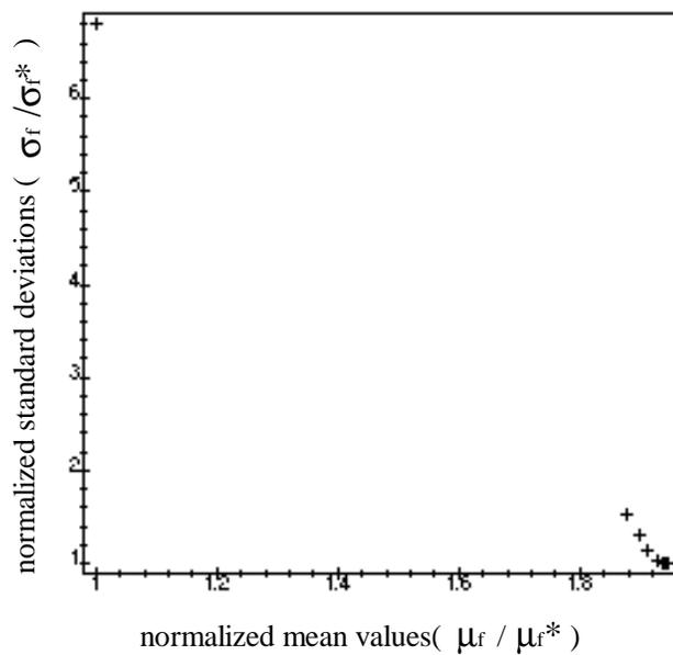
**Figure 5 Efficient Solutions Using the WS Method**
