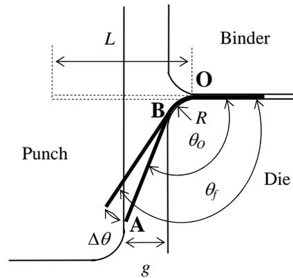
Figure 6. Schematic of a straight flanging process.
