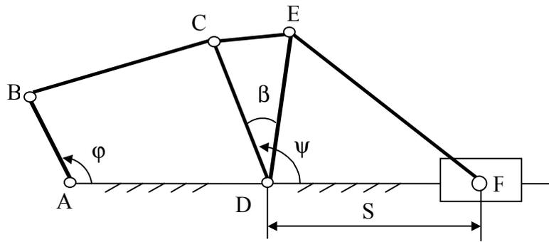
Figure 5. Six-link function-generator linkage
