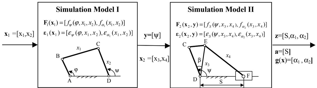
Figure 8 Simulation model for six-link function-generator linkage
