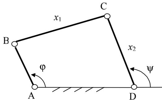
Fig. 6 The first four-bar linkage
